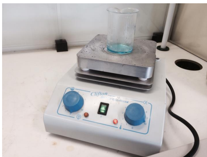
Figure 6. Digesting the brass sample for subsequent analysis.
