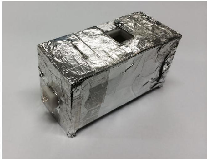
Figure 4. Colorimeter body covered with aluminium foil to improve light shielding.
